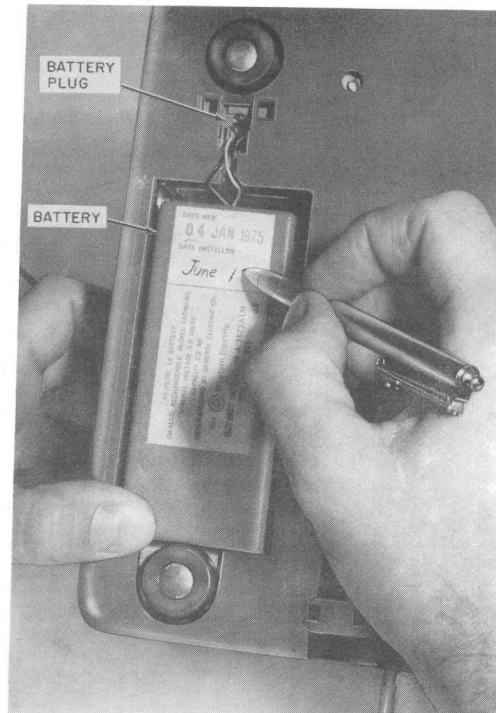
Fig. 6—870B1M or 2870B1M Dial, Partial Bottom View
